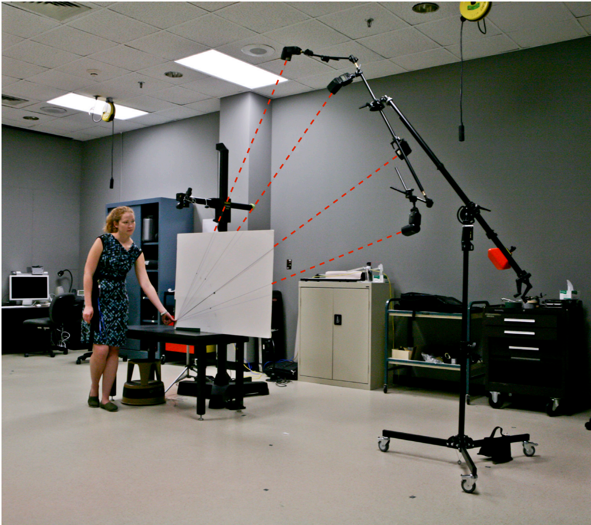
Figure 6 Webb calibrating the Mantis by pulling the four flash strings to the corner of the angle finder emphasized by the red dotted line. (The angle finder illustrated above is not the sweater dryer but is similar.)
