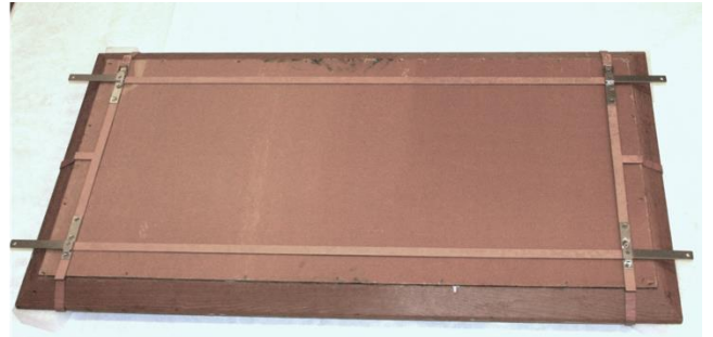
After integrating mounting system using Takiya folding bracket w/ d ring machine screwed to brass strip for hanging and securing to travel crate
