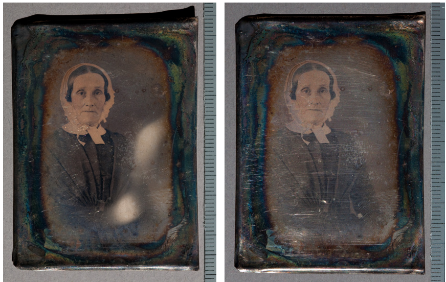
Figure 1 (left) The flare from the flash shows up towards the bottom right fogging some of the detail. Figure 2 (right) The snoot eliminates the stray light from the flash.
