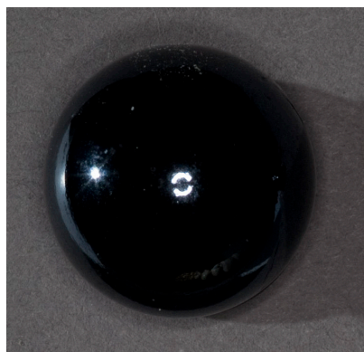
Figure 8 The reference sphere for the human skull RTI with the reflection of the ring light falling in the center. Before processing the image files, this center reflection from the ring light is removed.
